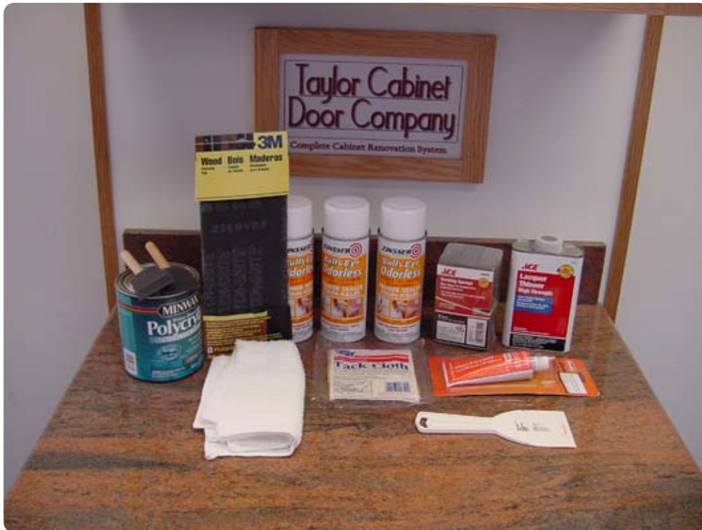
Materials for painting interior of cabinets
