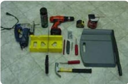
**The tools you'll need for the job.** There are only a few tools required for this project, most will be found in the average homeowners garage. You'll need: a jig saw, a hand miter box, a hammer, a screw gun, a tape measure, a paper cutter, a utility knife, a nail set, a pencil, a Phillips #2 screw driver, a small set of drill bits, some 3/4" finish nails and Contact Cement glue.
