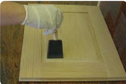
4. ***Open the can of Polyurethane and stir only!*** Starting with the back of the door first, apply the polyurethane evenly from the inside out, brushing in the direction of the grain.
