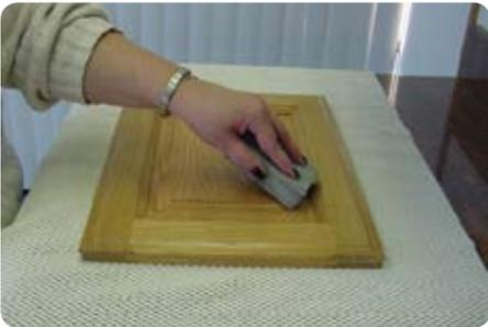
7. After allowing the door to dry completely (24 hrs), lay down the sanding mat and sand both sides of the door with a fine sanding sponge block.
